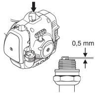
**CAUTION!** Always use the recommended spark plug type! Use of the wrong spark plug can damage the piston/ cylinder. Check that the spark plug is fitted with a suppressor. Ask your dealer or Husqvarna should you need more information.
