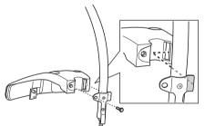
• Fit the dust cup on the shaft. The nut must be completely covered by the dust cup.
